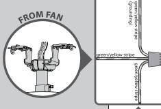
Using an orange wire connector from the \* hardware bag, connect the three grounding wires (green, green/yellow stripe, or bare copper) downrod, and hanging bracket.
