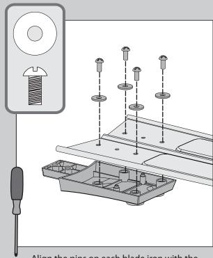
Align the pins on each blade iron with the appropriate pin holes on each blade. Secure the blade to the blade iron using the blade screws, found in the ▲ hardware bag, and blade washers, found in the ■ hardware bag.
