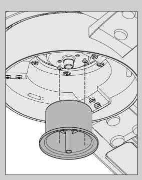
Wrap keyhole slots in the finial mount around the screws and twist counterclockwise.
