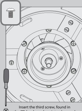
the hardware bag, into place and tighten all three screws.
