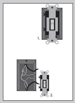
Shut off power to the room you will be working in at the breaker box. After removing the switch plate cover, remove all wiring from the switch.
