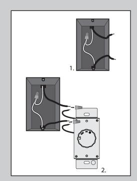
Using the wire connectors, connect each black wire from the wall control to a black wire from the switch box.
