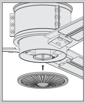
Screw the finial onto the threaded rod found at the bottom of the finial mount.
