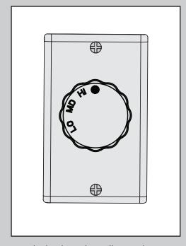
The knob on the wall control unit controls power to the fan. The fan has four speed settings in sequence: high, medium, low and off.
