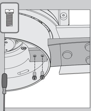
Insert each blade iron through a slot in the motor housing. Align the screw holes and install two blade iron screws, found in the X hardware bag, then securely tighten after both screws are attached.
