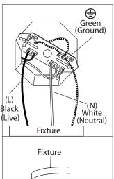
4. Tuck electrical wires into electrical box and position fixture over studs on mounting
