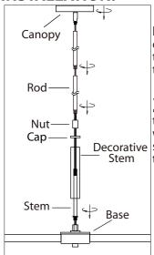
$\mathbb{1}_{\circ}$  Install the stem onto the base. Slide the decorative stem onto the screw stud. Tighten the cap against the assembly by the nut.
