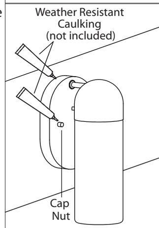
**7.** After installation, seal around the top and side perimeter between the fixture and the wall surface with weather resistant caulking. The bottom should be left un-caulked to prevent moisture build-up. Apply a small amount of weather resistant caulking around the side perimeter between the cap nut and mounting plate.
