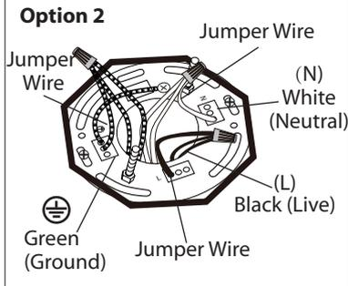
**Option 2:** For multiple green (ground), black (live) and white (neutral) wires joined in the electrical box (house wiring), attach a single "green", "black" and "white" jumper wire before connecting. Strip 7mm from the 6" jumper wires supplied. Then connect (push) wires into the correct inserts.
