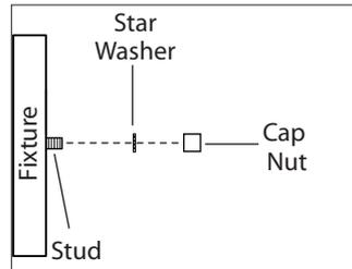
**4.** Tuck electrical wires into electrical box and position fixture over studs on mounting bracket assembly. Secure fixture in place with star washers and cap nuts.
