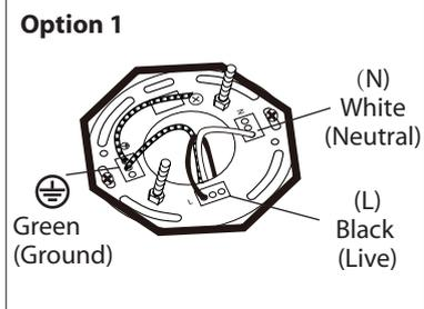
**2. Option 1:** Connect (push) electrical wires from electric box (house wiring) into correct inserts.
