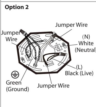
**Option 2:** For multiple green (ground), black (live) and white (neutral) wires joined in the electrical box (house wiring), attach a single "green," "black" and "white" jumper wire before connecting. Strip 7mm from the 6" jumper wires supplied. Then connect (push) wires into the correct inserts.
