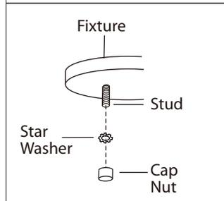
**4.** Tuck electrical wires into electrical box and position fixture over studs on mounting bracket assembly. Secure fixture in place with star washers and cap nuts.
