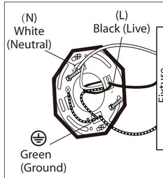
**3.** Connect (push) electrical wires from fixture into correct inserts.
