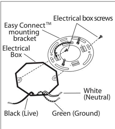
**1.** Attach Easy Connect<sup>™</sup> mounting bracket to electrical box with electrical box screws (not included).
