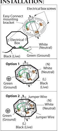
$\mathbb{1}_{ extstyle \circ}$  Attach easy connect mounting bracket to electrical box with electrical box screws (not included).
