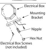
$\mathbb{Z}_{\circ}$  Attach the mounting bracket to the electrical box using electrical box screws (not included). Attach the nipple to the mounting bracket and adjust until it will clear the canopy when assembled (Place the canopy over the nipple and tighten the upper connector onto the nipple until snug. The upper connector should hold the canopy snug to the ceiling). Lock the nipple in the correct position using the hex nut.
