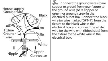
$igotimes_{\circ}$  Once connections of wires are completed, carefully tuck wires and wire nuts into the electrical box making sure no bare wire (on the black and white) is visible at the wire nuts. Slide canopy into position and tighten in place by nut into position.
