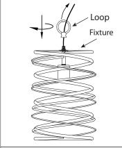
$\mathbb{1}_{\circ}$  Tighten the loop to the stem on the fixture.
