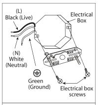
1 o Attach easy connect mounting bracket to electrical box with electrical box screws (not included).
