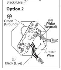
**Option 2:** For multiple black (live) & white (neutral) wires joined in the electrical box (house wiring), attach a single "black" and "white" Jumper Wire before connecting. Strip 7mm from a 6" Jumper Wires (AWG 12-24) supplied. Then connect (push) wires into correct inserts.
