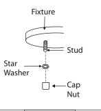
Tuck electrical wires into electrical box and position fixture over studs on mounting bracket assembly. Secure fixture in place with star washers and cap nuts.
