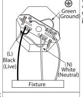
3. Connect (push) electrical wires from fixture into correct inserts.
