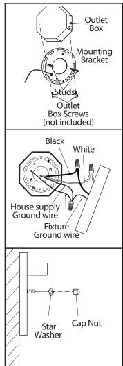
**1** Mount the mounting bracket to outlet box using outlet box screws (not included). Make sure the studs on the mounting bracket are facing out from the outlet box.
