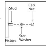
Tuck electrical wires into outlet box and position fixture over studs on mounting bracket assembly. Secure fixture in place with star washer(s) and cap nut(s).
