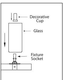
Position glass on the fixture and push into place. Insent the decorative cup onto the socket.
