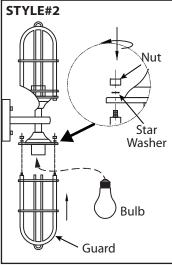
**STYLE#2** - Install specified bulb type and wattage. Install the guard with star washers and nuts.
