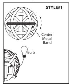
**STYLE#1** - Press and turn the center metal band to leave space. Install specified bulb type and wattage.
