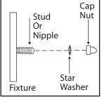
Tuck electrical wires into outlet box and position fixture over studs or nipple on mounting bracket assembly. Secure fixture in place with star washer(s) and cap nut(s).
