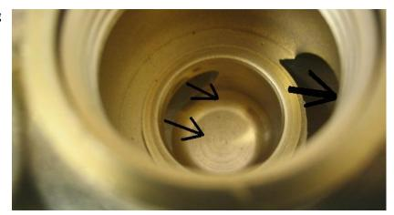
**Photo 3** – shows top view of valve body indicating water flow direction as related to body's ports and passage ways.
