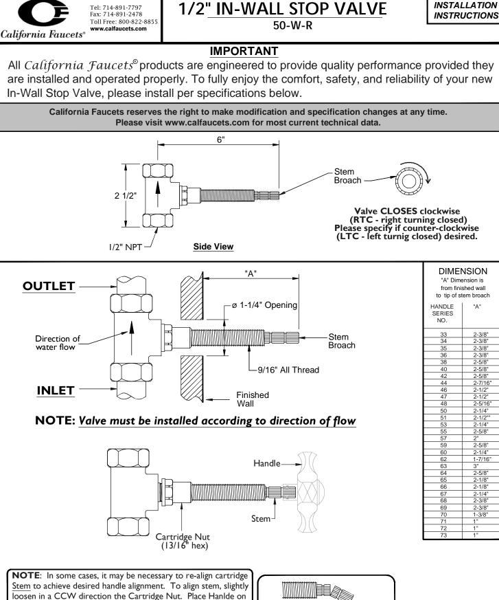
Stem and **TIGHTEN** in a CW direction until desired alignment of handle is acheived. Retighten <u>Cartridge Nut</u> to factory torque setting of 14 ft-lbs. (Cartridge Nut size is 13/16" hex) **WARNING**: <u>Cartridge Nut</u> **MUST** be propler torqued to prevent possible failure and/or water damage.
