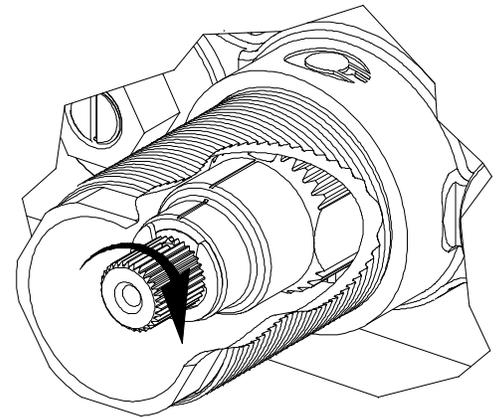
Rotate CW for Cooler (shown)
