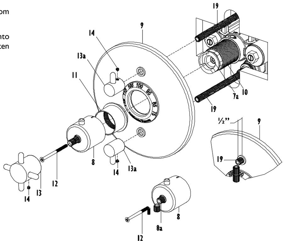
The thermostatic cartridge has built-in screens to prevent debris from affecting proper operation of anti-scald protection. Debris may build up on screens this will affect water flow and will require occasional service.
