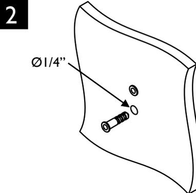
Drill holes and press in anchors
