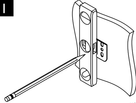
Mark location of holes using wall mount and level
