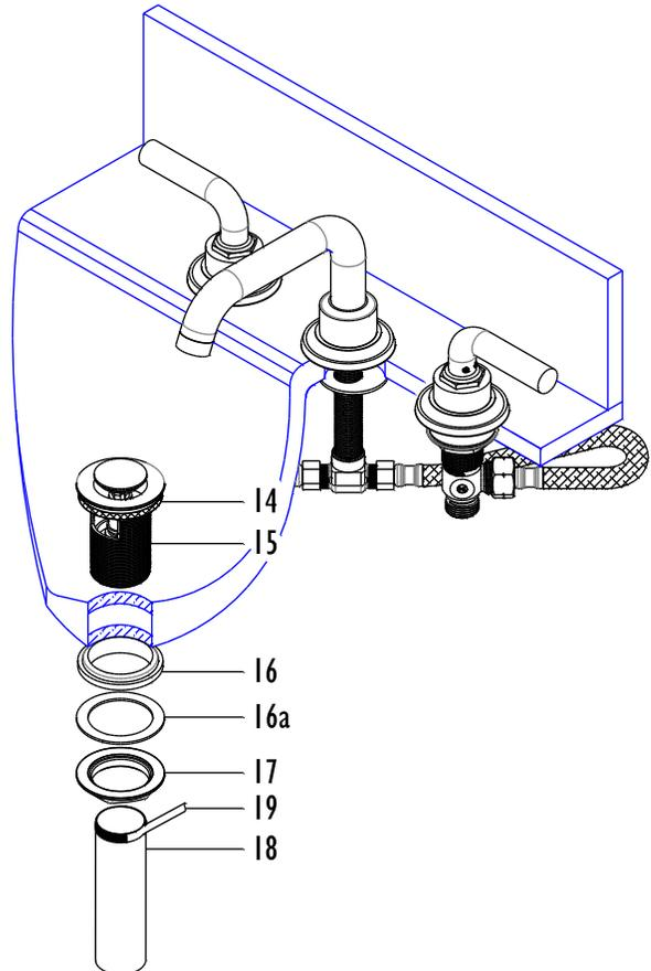
**IMPORTANT:** Prior to attachment, flush supply lines to remove debris that may cause damage or malfunction to valve cartridge.
