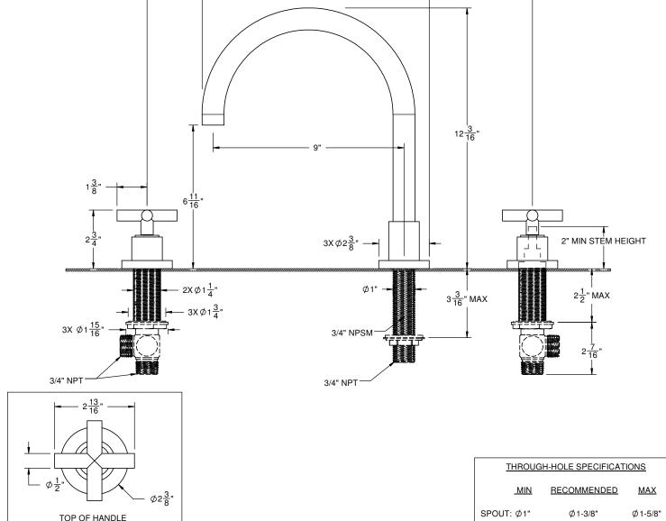
SPOUT: Ø1" Ø1-3/8" Ø1-5/8" VALVE: Ø1-1/4 " Ø1-3/8" Ø1-5/8"
