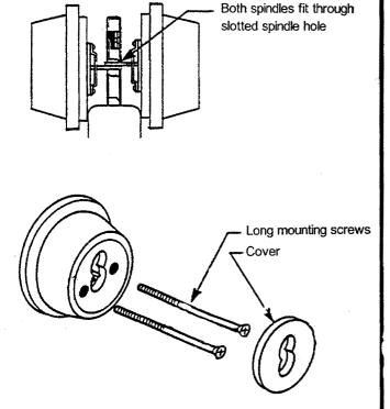
Note 1: Mount cylinders on the doors so that the mounting screws enter from the inside of the door.
