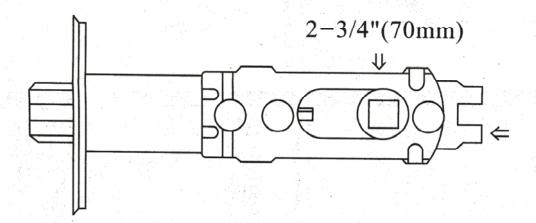
THE LATCH IS SET 2-3/4"(70mm) TO ADJUST TO 2-3/8"(60mm) PULL IN THE REAR PART
