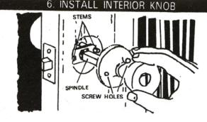
Install interior knob and rose by placing on spindle and aligning screw holes with stems push flush against the door insert screws and tighten until lockset is form
