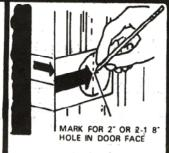
Mark center hole on door face through guide on template for 2-3 8" 2-3 4".
