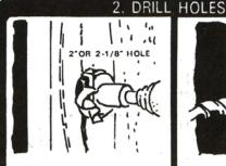
Drill 2" or 2-1 8" hole through door face as marked for lockset It is recom mended that holes be drilled from both sides to prevent splitting.
