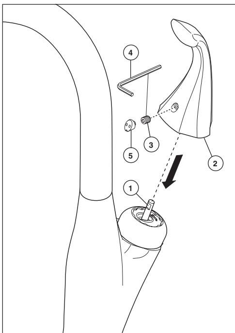
Making sure the flat of valve stem (1) is facing the set screw hole of handle (2), slide handle (2) over valve stem (1) until it
