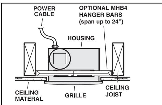
To mount housing anywhere between joists, i-joists or trusses, use optional hanger bar kit MHB4 (sold separately). Follow mounting instructions included with kit.
