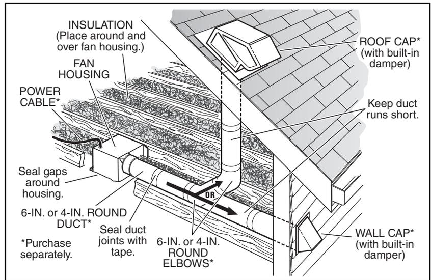
The ducting from this fan to the outside of the building has a strong effect on the air flow, noise and energy use of the fan. Use the shortest, straightest duct routing possible for best performance, and avoid installing the fan with smaller ducts than recommended. Insulation around the ducts can reduce energy loss and inhibit mold growth. Fans installed with existing ducts may not achieve their rated airflow. 6" round metal duct is recommended for best performance.
