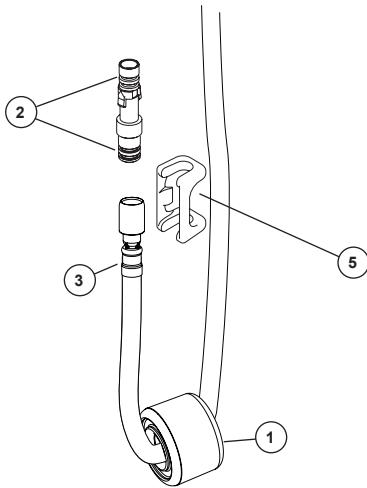
Slide weight (1) onto pull down hose (3). Lubricate (lubricent included) o-rings on adapter (2), insert adapter into pull down hose (3). Connect clip (5) to secure adapter.
