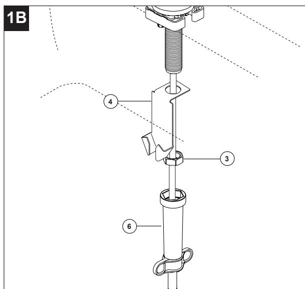
Place bracket (4) on spout shank. Slip nut (3) over spout shank and secure with mounting wrench (6).
