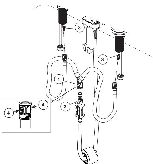
Install quick connect hose assembly into bracket and attach to end valve nipples (3). Snap the pull down hose and adapter (2) to Y connector hose fitting (1). Pull down moderately to ensure each connection has been made.
