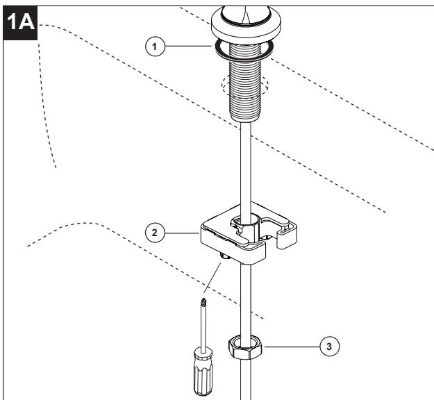
**NOTE:** When drilling mounting holes for the spout, it is recommended that the hole size be 1 1/4" to 1 1/2".
