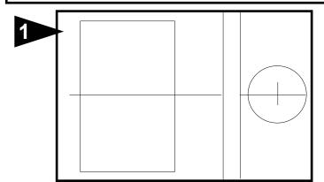
Select location on vertical surface of warm or return air plenum for mounting humidifier. Tape mounting template in place making sure the template is level. Do not install humidifier or 6" bypass pipe where the blanked off ends of a cooling coil will restrict air flow to the humidifier. Extend horizontal centerline from template to the adjacent plenum. Scribe 6" circle 10" to 15" from side of humidifier, on cabinet centerline, using connecting collar as guide.
