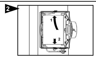
Cut out center section of template and 6" hole. Humidifier is self retaining. Slide top side in first, then slide chassis down. Level chassis and install center screws. If by-pass pipe installs to opposite side of chassis, bend clip on chassis, remove side discharge, and reinstall discharge to opposite side of chassis. Install remaining four corner screws.
