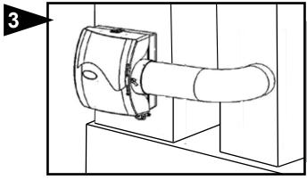
Connect by-pass pipe to collar and humidifier cabinet. Using holes at top and bottom of side panel discharge, pierce 2 self tapping screws through by-pass pipe.
