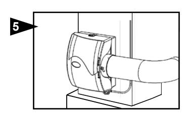
Connect 1/4" water supply tube to brass filter at inlet of solenoid. DO NOT USE PLASTIC TUBING IN CONTACT WITH ANY HOT PLENUM SURFACE OR DUCT. IF USING PLASTIC TUBING, USE INSERT FOR PLASTIC TUBING AND PLASTIC COMPRESSION SLEEVE (INCLUDED WITH SADDLE VALVE KIT).
