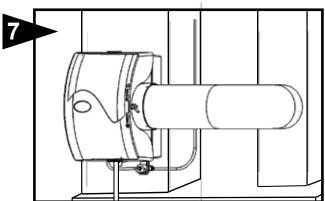
Connect drain hose to 1/2" spout on humidifier cabinet using hose clamp. Run 1/2" hose to suitable drain such as floor drain, sewer or laundry sink. Be sure hose has continuous slope and is not kinked at any point.
