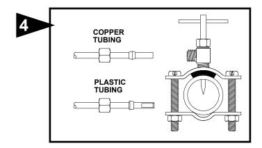
Mount the self tapping saddle valve on either a cold or a hot water pipe. A side or top mount is best to avoid clogging from pipe sediment. Connect 1/4" O.D. tubing to the saddle valve. Copper tubing requires a brass compression nut and brass sleeve. Plastic tubing requires a brass insert inside the tubing and a plastic sleeve on the outside with a brass compression nut.
