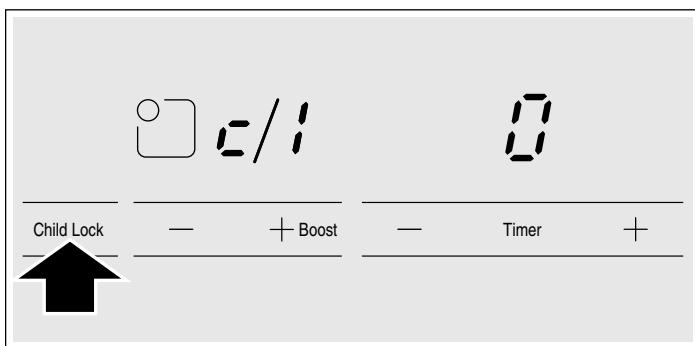
3. Touch the **Child Lock** key until the indicator for the required function is displayed.
