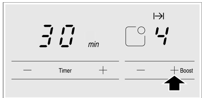
4. Touch the **+** or **-** key to set the desired time. After a few seconds the timer will start to count down.
