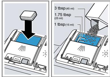
If you are using tablets, one is enough. Insert the tablets in a horizontal position. If you are using powder or liquid detergent, follow the manufacturer's instructions and quantities for dosage in the detergent dispenser. 1.5 to 1.75 Tbsp (20 ml – 25 ml) detergent is sufficient for normal soiling. If dishware is only lightly soiled, slightly less than the amount of detergent specified is usually sufficient.
