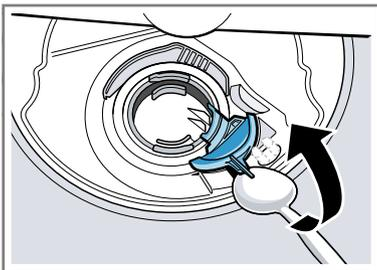
6. Lift the pump cover diagonally inward and take it out.
