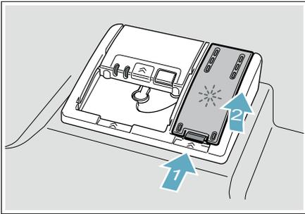
2. Add liquid rinse aid to the dispenser [31] until it is full. Do not overfill. Avoid spilling into air vent hole.
