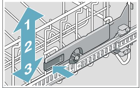
4. To **lift** the upper rack; grip the sides of the upper rack along the upper edge and lift.
