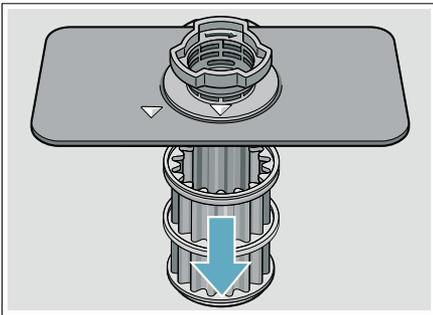
3. Rinse the filters under running water and use a soft brush to clean.
