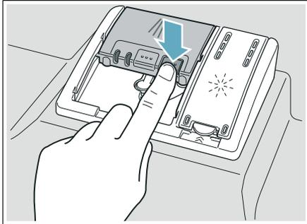
2. When using detergent tabs, lay them such that they do not come in contact with the cover, insert a detergent tab flat, not on its side.
