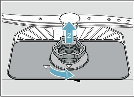
2. Remove the microfilter from the fine filter for easier cleaning.
