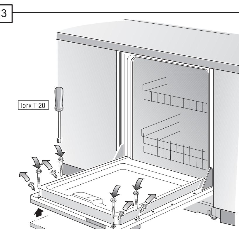
Remove shipping screws and replace with screw ③.
