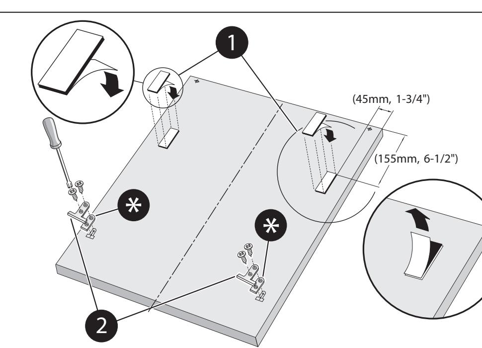
If your unit came with a rubber apron, you will need to use the plastic spacers ③ during your Fully Integrated panel installation. Place one plastic spacer between each metal bracket and the panel, if required. Attach the metal brackets ② (and plastic spacers if necessary) as shown. Install the hook and loop fastener strips ①, exposing adhesive on both sides of each strip.
