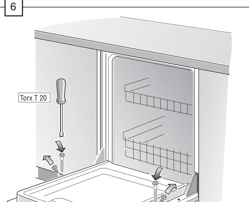
Remove shipping screws and replace with screw ③.
