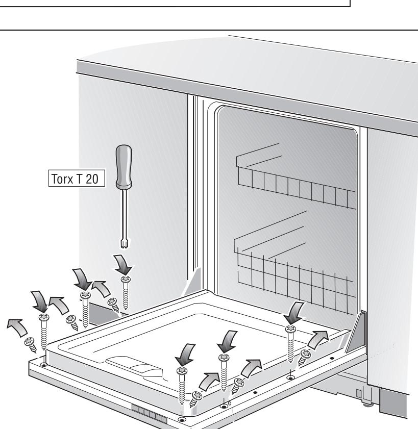
Remove shipping screws and replace with screw ③.
