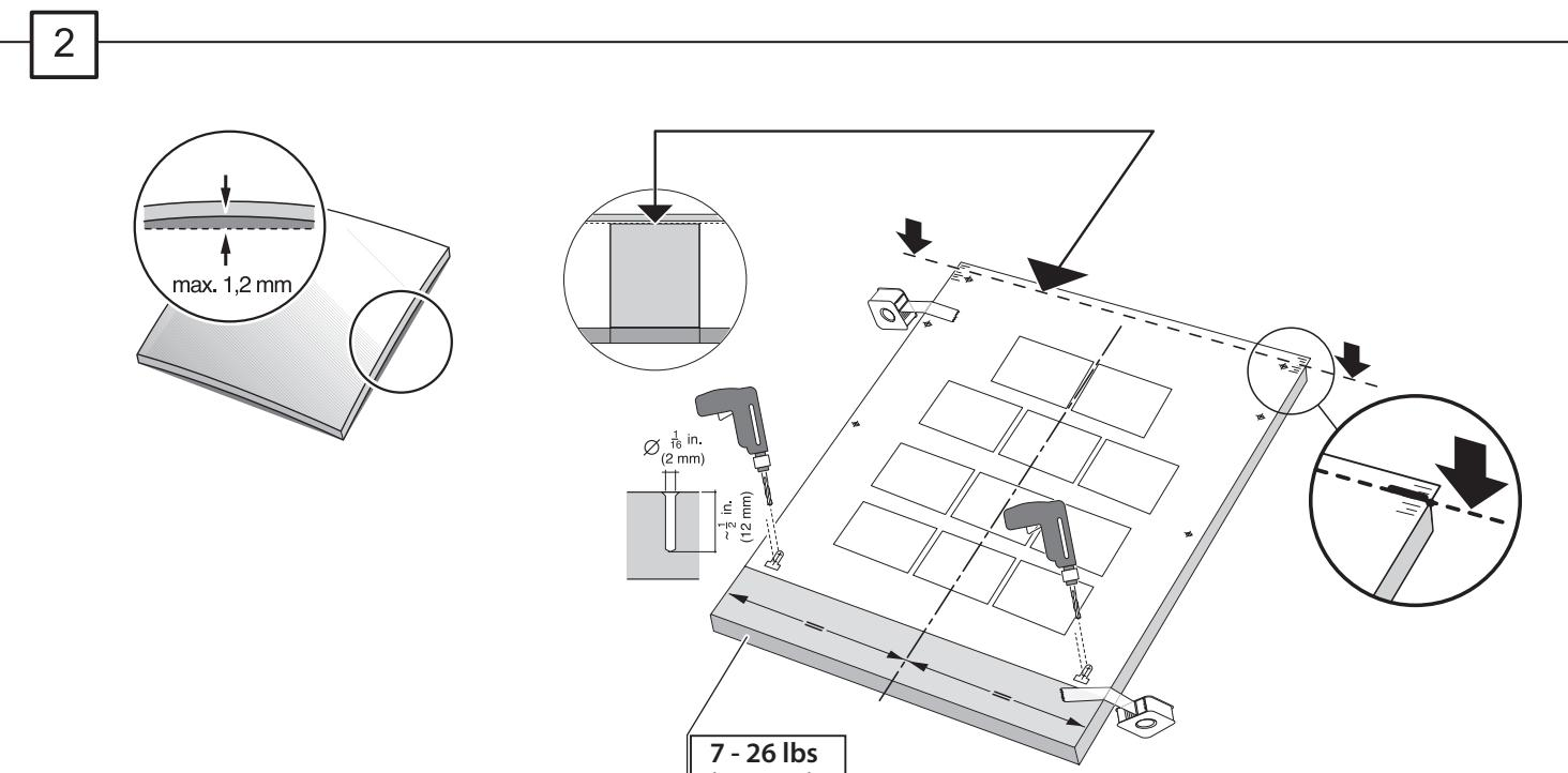
Tape marked template to door panel, being sure to align marks with top of top cabinet piece. Then using drill start holes for screws ②. DO NOT drill completely through door!!
