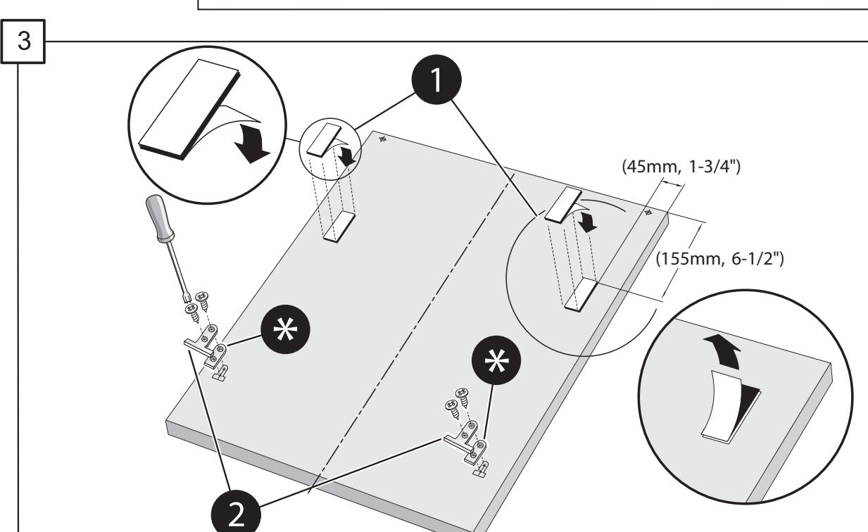
If your unit came with a rubber apron, you will need to use the plastic spacers ③ during your Fully Integrated panel installation. Place one plastic spacer between each metal bracket and the panel, if required. Attach the metal brackets ② (and plastic spacers if necessary) as shown. Install the hook and loop fastener strips ①, exposing adhesive on both sides of each strip.
