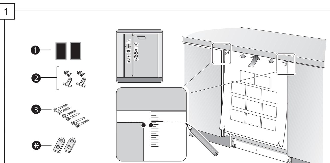
Place door template on door, making sure correct side is up. Slide template up, until it butts against bottom of counter. Then mark height of adjacent cabinet door as shown.
