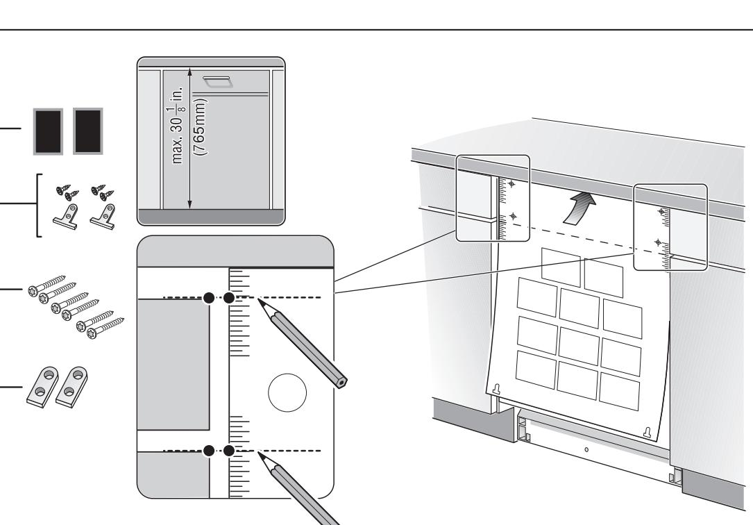
Place door template on door, making sure correct side is up. Slide template up, until it butts against bottom of counter. Then mark height of adjacent cabinet door and drawer as shown.
