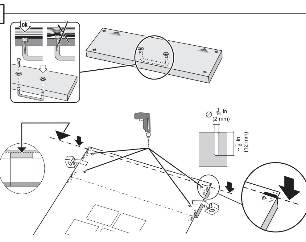
Tape marked template to drawer panel, being sure to align marks with top of top cabinet piece. Then using drill start holes for screws ①. DO NOT drill completely through cabinet!!!
