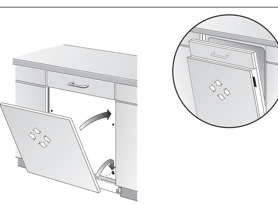
Insert metal mounting brackets at bottom of door. Then press the top of the door to attach to the dishwasher. Position door as necessary.
