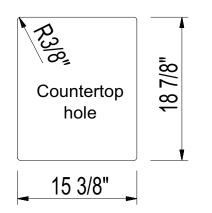
**NOTES:** Refer to installation instructions supplied with kitchen sink for undermount, or drop-in installations. Templates and installation kits provided with the sink.
