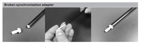
If a synchronization adapter is broken, it can easily be replaced by simply sliding another in its place.
