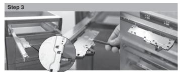
Carefully remove the synchronization rod. Repeat these steps on the remaining drawers.
