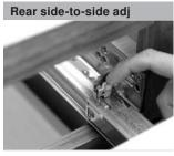
Rotate the rear side-to-side adjustment left or right to re-align the back of the drawer box with the front.
