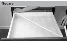
Check drawer box squareness, either by measuring from inside corner to inside corner, or by using a framing square.
