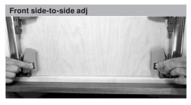
Rotate side-to-side adjustment left or right equally on both locking devices. Drawer front moves in the same direction as rotation.
