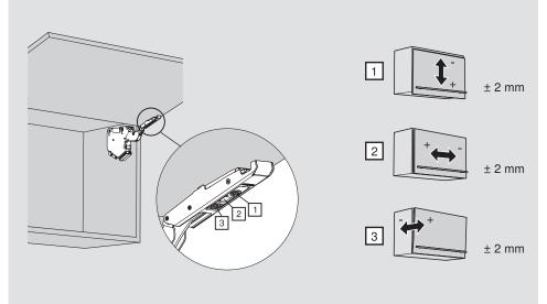
Use a POZI screwdriver on cam adjustments for each of the three 3-dimensional adjustments.
