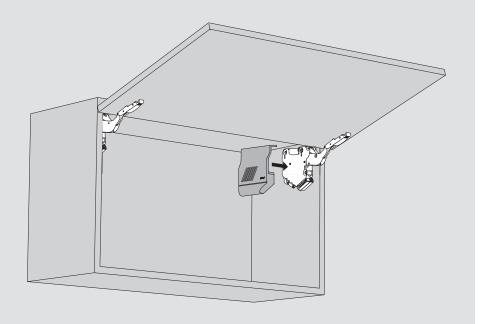
Place the left and right cover plates over the appropriate lift mechanisms and snap them in place.
