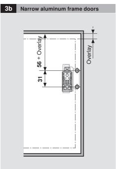
NOTE: Attach each mounting plate with two 606N or 606P wood screws for wood doors, two 7072A screws for wide aluminum doors or two 699.110 screws for narrow aluminum doors
