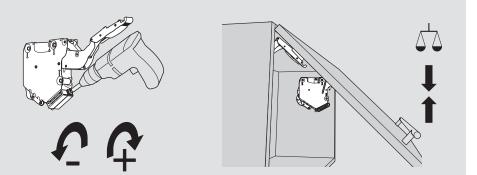
Use a screw gun, POZI driver bit insert and bit holder to adjust each lift mechanism to the desired tension.
