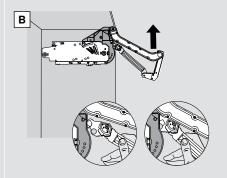
Lift up on the arm assembly to lock into place.
