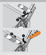
After cutting the rod to size, slide the stabilizer arm cover caps onto the rod. Insert the stabilizer rod adapters being careful to line up the tabs (shown with dotted lines). Attach the rod assembly to each arm assembly and tighten the locking screw.
