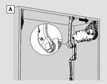
Attach the arm assembly to the lift mechanism as shown in illustrations A and B.
