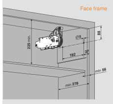
NOTE: Face frame cabinets must be blocked out flush with the frame
