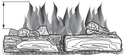
Figure 34 - Incorrect Burner Flame Pattern
