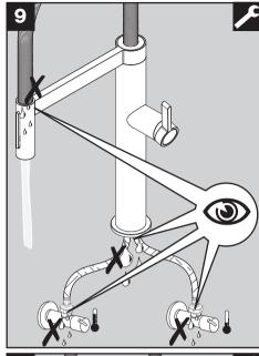
Double check all connections for leaks.
