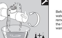
Before connecting supply lines to the water valves, flush each water valve to remove dirt and particles that can affect the functioning of the faucet and void warranty.
