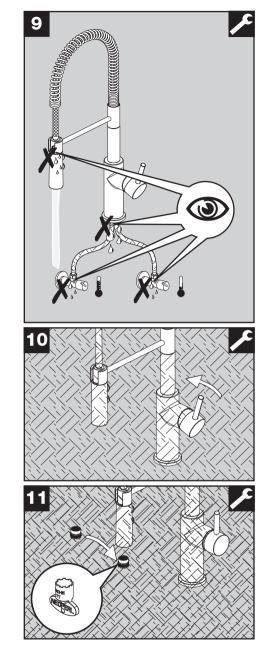
Double check all connections for leaks.
