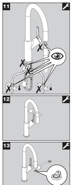
Double check all connections for leaks.
