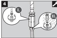
Connect spray hose (9) to outlet hose (13) with rubber washer in the connection (14).
