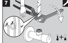
Connect red supply line to hot water valve and blue supply line cold water valve.
