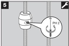
Attach weight (16) to spray hose using screws provided.
