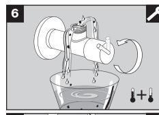
Before connecting supply lines to the water valves, flush each water valve to remove dirt and particles that can affect the functioning of the faucet and void warranty.
