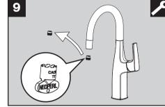
Remove aerator using the aerator key (12).
