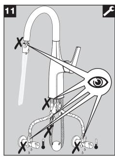
Double check all connections for leaks.
