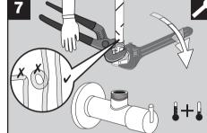
Connect hot supply line (red) and cold supply line (blue) to hot and cold water valves.
