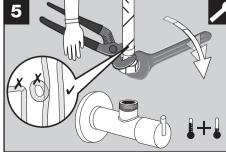
Connect red supply line (12) to hot water valve and blue supply line (13) to cold water valve.
