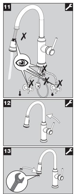
Double check all connections for leaks.
