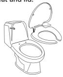
Remove mounting bolts to release existing toilet seat from the toilet.
