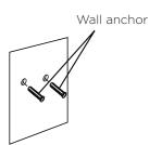
2. Install the wall anchors in the newly drilled holes.
