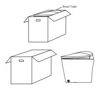
1. Open the box right side up. Remove the accessories first, then remove the unit from the top as shown in the diagrams above.
