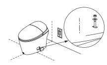
3. Secure the toilet base. Press down evenly on the toilet to set the wax ring. Install a washer and nut onto each bolt. Hand tighten the nuts. Use a wrench to tighten the nuts one quarter turn beyond hand tight.
