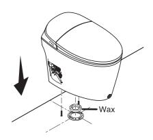
2. Place the wax ring and toilet base and position the wax ring on the flange. Remove the access covers and cap from the water inlet on the back of the toilet. Align the toilet over the flange and bolts. Carefully lower the toilet into the flange.
