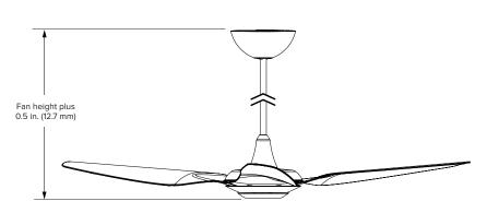
The Haiku Fan Light Kit adds 0.5 in. (12.7 mm) to the total fan height. See the Haiku fan spec sheet for exact fan heights, which depend on the fan's mount, diameter, and other factors.
