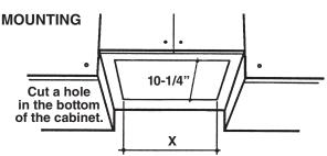
X = 19-1/2" for P195P1M52SB6 X = 26-5/8" for P195P1M70SB6
