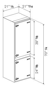
The refrigerator is installed on the cabinet base shelf and not on the kitchen floor.
