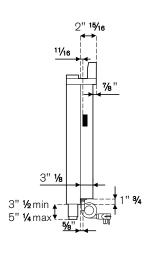
Bertazzoni recommends to operate the appliance after it has been installed in a cabinet. The kitchen cabinets shall be made of materials capable of withstanding temperatures at least 117°F (65°C) above room temperature in order to avoid possible damage to the cabinets during oven usage. For further installation instructions refer to the installation manual.
