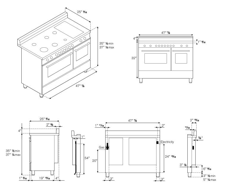
Bertazzoni recommends to operate the appliance after it has been installed in a cabinet. The kitchen cabinets shall be made of materials capable of withstanding temperatures at least 117°F (65°C) above room temperature in order to avoid possible damage to the cabinets during oven usage. For further installation instructions refer to the installation manual.
