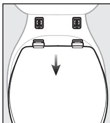
**Pull seat forward to disengage and remove.**
