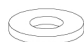
N x8 Flat Washer \phi 5/16" x16x2mm * x8 Rondelle plate \phi 5/16" x16x2mm x8 Arandela plana \phi 5/16" x16x2mm
