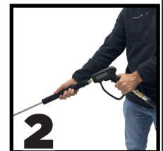
2 Purge water from system.
