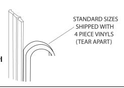
**9** Once the **Glass Panel** is set in place, cut two pieces of the **Vinyl** 1/2" longer than the exposed glass. Cut both ends of each **Vinyl** square so it will sit tight against the side of the **Wall Jamb**.
