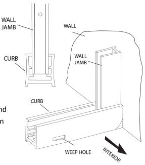
**5** Wipe the shower walls, sill, **Curb** & **Wall Jambs** with a clean, dry cloth to remove any dust or debris. Apply a 1/4" bead of silicone along the inside of the pencil lines that were marked in Step #3. Carefully place the **Curb** on the sill, over top the silicone, in the position marked. BE SURE THE WEEP HOLES FACE THE INTERIOR.
