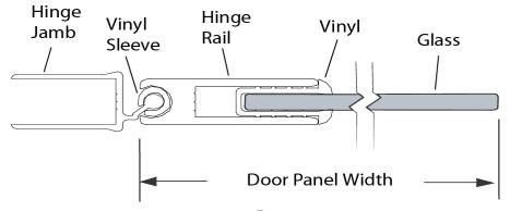
**8** The glazing **Vinyl** for this door are designed to fit tightly between the glass and metal frame.
