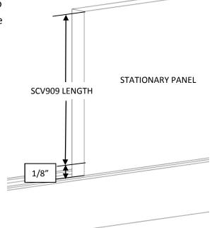
**11** With a helper inside, slide the **Hinge Jamb** over the **Wall Jamb**, the flush side of the **Hinge Jamb** and **Hinge Rail** will be at the top. While keeping the **Hinge Jamb** over the **Wall Jamb**, align the **Door Panel** and **Vinyl** so there is a continuous 1/8" gap. TIP: Put an 1/8" **Setting Block** between the **Door Panel** and **Vinyl** to help with the alignment.
