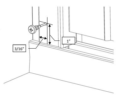
14 Install the Latch to the Door Panel by placing the Latch Vinyl on the glass first , then pressing the latch over top of the Vinyl. Be sure to install the Latch directly in the middle of the the two holes in the Door Panel. Carefully cut any excess vinyl not covered by the Latch.
