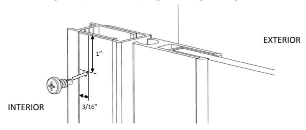
13 After the top Screw is in place, install another Self Drilling Screw into the bottom of the Hinge Jamb and Wall Jamb 1" above the Curb and 3/16" from the edge of the open side of the Hinge Jamb (see illustrations), being sure it also goes through the Wall Jamb.
