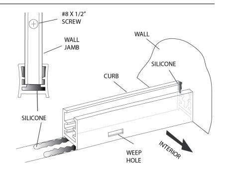
**6** The **Glass Panel** must be 1/4" into the **Wall Jambs**. To aid in setting the **Glass Panel**, place a piece of tape at the top and bottom of the **Glass Panel** 1/4" from the edge on the side that will go into the **Wall Jamb**. If the edge of the tape is exposed, the **Glass Panel** is not seated far enough into the **Wall Jamb**.
