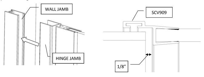
**12** Once the **Vinyl** is aligned and the **Hinge Jamb** is over the **Wall Jamb**, inside of the shower insert one of the **Self Drilling Screws** into the **Hinge Jamb** about 1" from the top and about 3/16" from the edge of the open side of the **Hinge Jamb** (see illustrations), being sure it also goes through the **Wall Jamb**.
