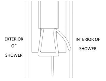
**20** Install the **Drip Vinyl** so it is flush against the **Glazing Vinyl** on the **Hinge Rail**. Close the door until it rests against the **Glass Panel/SCV909 Vinyl**. Notice where the **Drip Vinyl** lines up with the **SCV909 Vinyl** and cut the **Drip Vinyl** flush (Illustration Below).
