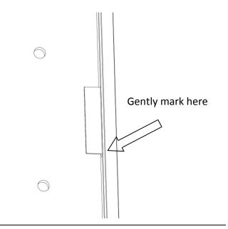
**16** Reinstall the bottom half of the **Insert** to **Vinyl** and then install the **Magnet** and finally the last piece of the **Insert**. The **Magnet** should line up with the **Latch** when installed, adjust if necessary.
