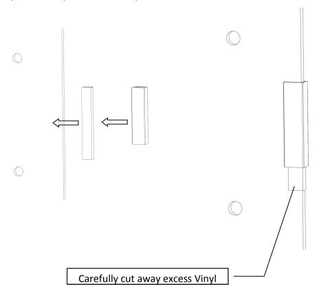
**15** Close the **Door** into the **Strike Vinyl** and gently mark on the **Strike Jamb** where it meets the bottom of the **Latch**. Remove the **Strike Vinyl** and take out the smaller insert of the **Vinyl**. Cut the insert at the marked height. Then cut 3" off of the top portion of the **Insert**.
