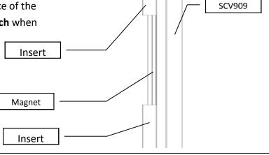
**17** While the **SCV909 Vinyl** is removed, measure the length between the **Hinge Jamb**, and the **Panel Glass** and subtract 1/16". Cut the **Curb Filler** to this length.
